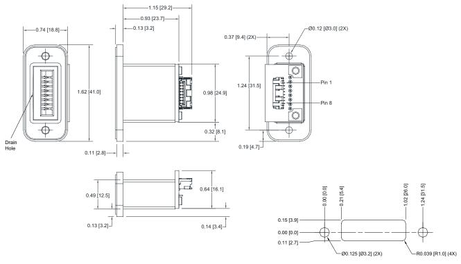
**Installation Recommendation**: For best water drainage, it is recommended that the receptacle be installed with the output connector above the housing as shown above.
