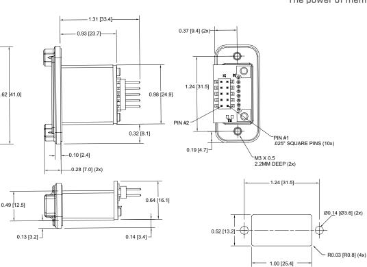
Installation Recommendation: For best water drainage, it is recommended that the receptacle be installed with output connector above the housing as shown above. Note: Installation screws are supplied by the customer.
