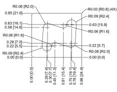
MOUNTING SURFACE REQUIREMENTS:  $\boxed{\bigcirc 0.005}$  AND  $\stackrel{32}{\sim}$
